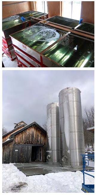
**FIGURE 6.43.** Transfer and storage tanks for sap come in a wide variety of sizes and configurations and should be food-grade, clean, and suitable for intended use.
