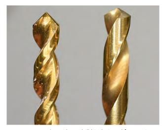
**FIGURE 6.5.** A clean, sharp drill bit designed for tapping maple trees (left) is different from a standard wood bit (right). Tapping bits are made for rapid cutting of fresh wood in live trees and fast removal of wood chips from the taphole. Bits should be replaced if damaged or after about 2,500 tapholes.
