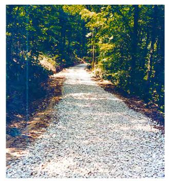
**FIGURE 5.28.** As a general rule, producers are advised to avoid developing large, heavily compacted, graveled roads in the sugarbush. Exceptions to this would be the need for a main road to the sugarhouse to support delivery or transport vehicles or customers in passenger cars. Under those circumstances, both the main road and the parking areas around the sugarhouse should be finished for access in all types of weather and conditions."
