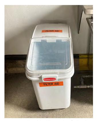
**FIGURE 8.6.** Filter aid should be stored in a food-grade container with a lid so it remains dry and clean for use.
