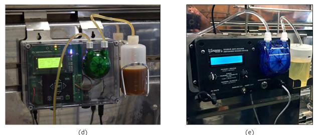
**FIGURE 7.12.** Several types of methods are available to disperse foam, from manual droppers (a), to passive cups filled with defoamer that hang over the pan edge in the evaporator (b), to liquid droppers (c), or fully-automated systems (d and e) that dispense defoamer both on a timed and as needed based upon a foam detecting probe.
