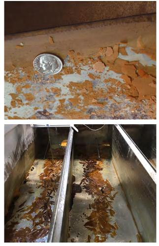
**FIGURE 7.14.** Niter (nitre) in evaporator pans. Niter that is attached is termed "scale" while niter that has flaked off and broken into small pieces and carried along in syrup is called "sugar sand." Dime for scale.
