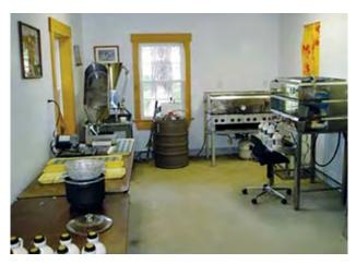
**FIGURE 9.2.** A spacious, clean, ordered, well-equipped area is desirable for making and packaging maple products. Equipment visible includes container and basket for crystal coating candy (left front), soft sugar candy machine with molds (left middle), maple cream machine (left rear), syrup barrel (rear center), propane-fired syrup reheating pan (right rear), canister pressure filter (right middle on floor), and syrup canning equipment (right front). (OBER)
