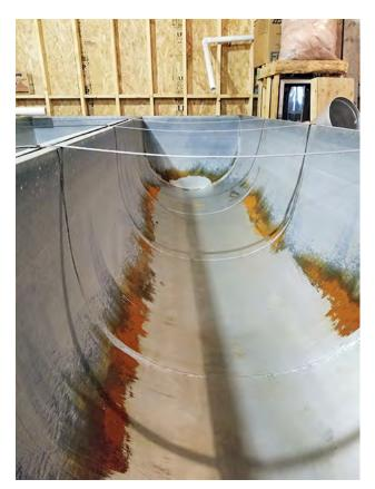
**FIGURE 14.5.** Equipment used for sap collection and storage and for syrup production and storage should be clean, lead-free, and undamaged. This tank is unsuitable and should be retired.
