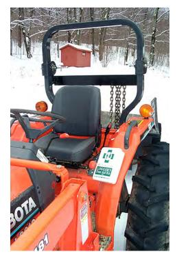
**FIGURE 13.4.** Every tractor and motor vehicle should have a first aid kit. Tractors should always be equipped with a roll-over protective structure.
