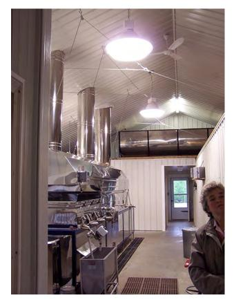
**FIGURE 12.15.** Cables attached to a beam or collar ties can be used to relieve stress on the evaporator from the weight of a "piggyback," Steam-Away<sup>®</sup>, or other evaporator accessories.
