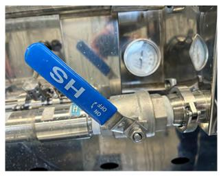
**FIGURE 7.16.** A partially-closed valve positioned between the pan and the draw-off valve can be used to help regulate the flow of syrup at the draw-off and to prevent the liquid level from dropping too low in the syrup pan.
