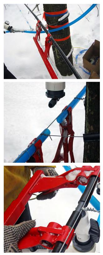
**FIGURE 6.29.** Mainline installation tool, which grips the tubing (top) and holds it in place while it is cut (center), then pushes the tubing over both sides of the fitting by turning a crank that closes the tool (bottom).
