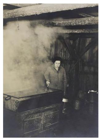
**FIGURE 2.12.** Katherine Skinner boils on a continuous flow evaporator on a metal frame wood-fired arch in Westmore, Vermont, in the 1940s. (GAUTHIER)
