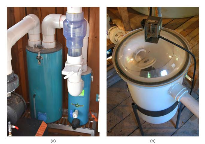
**FIGURE 6.37.** Moisture (also called vapor) traps help to protect vacuum pumps from ingesting liquid that can cause damage. Two moisture traps used in series (a) and a larger single moisture trap (b).
