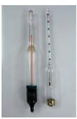
**FIGURE 7.17.** Hydrotherm (left) and hydrometer (right).
