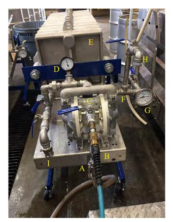
**FIGURE 8.8.** A plate filter press assembled and ready to filter syrup. This press is equipped with an air-powered diaphragm pump. Components include: unfiltered syrup inlet (a), air inlet (b), diaphragm pump (c), pressure gauge (d), plate press and papers (e), filtered syrup outlet (f), temperature gauge (g), filtered syrup sample port (h), and press bypass port (i).
