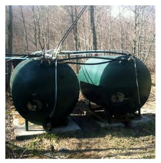
**FIGURE 6.39.** "Zero" tanks in which a vacuum is pulled serve as both extractor and sap storage. These tanks typically have a vacuum rated stamped on them. Exceeding this level can lead to tank collapse.
