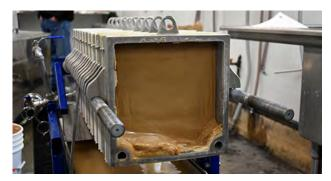
**FIGURE 8.7.** Cake of D.E., sugar sand, and syrup in a filter press after use. Inspection of the cake thickness in relation to the plate cavity will inform the producer of how much filtering capacity has been used in the filtering run.
