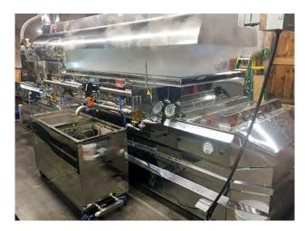
**FIGURE 7.5.** A modern maple evaporator designed for boiling high Brix concentrate, with cross flow pans and a reverse flow option to allow drawing off from one fixed position.
