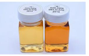
**FIGURE 8.18.** Temporary grading kits will lighten with exposure over time, making any grade determination incorrect.
