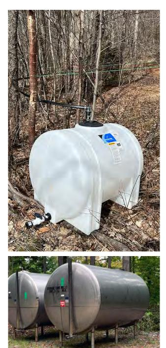
nonabsorbent, smooth, corrosion resistant, and able to withstand repeated cleaning and sanitation. Stainless steel, food-grade plastic, fiberglass, and glass meet these standards (**Figure 6.43**). Porous tanks, such as unsealed concrete, are not suitable as sap storage tanks. Galvanized tanks and tanks with lead solder or rust should not be used. It must be remembered that the evaporation process concentrates
