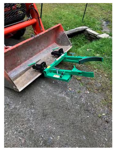
FIGURE 13.12. Use mechanical aids such as this barrel lift on a tractor to move heavy loads and prevent back injuries.
