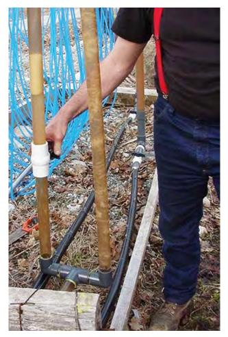
**FIGURE 6.41.** Pipe sap ladder in foreground. Producer has hand on shut-off valve that can be used to convert two pipe sap ladder to a single pipe sap ladder.
