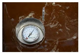
**FIGURE 8.14.** The Smokey Lake Maple Products Murphy Cup<sup>™</sup> or Murphy Float<sup>™</sup> has a built-in indication of the necessary correction of syrup density. These tools are used in conjunction with a hydrometer. In this example, the hydrometer should read 62.3°Brix for the syrup to be at the correct density.
