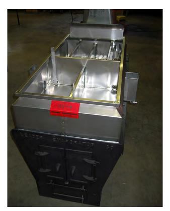
**FIGURE 7.1.** Basic components of a maple evaporator. The arch sits on the floor and contains the heat source (wood in this case). Pans sit upon the top of the arch and hold the boiling liquid. The stack (rearmost in photo) exhausts the excess heat and combustion gases safely out of the vicinity.
