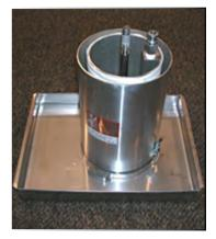
**FIGURE 8.9.** Inner and outer sleeves of a canister pressure filter showing filter cloth wrapped around inner canister. Lid and hoses are not shown.
