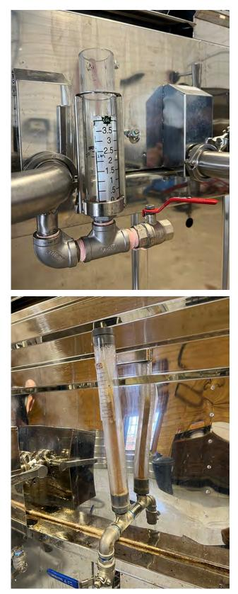
**FIGURE 7.11.** Liquid sight level indicators placed in both the front and back pans allow the operator to tell at a glance if there is a problem with sap/syrup depth.
