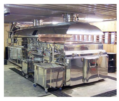
**FIGURE 11.4.** Sap must be processed into syrup quickly via boiling or reverse osmosis in combination with boiling.
